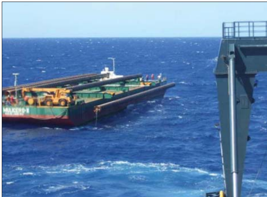
The 48-in. diameter conductors were launched from a barge and penetrated the soft bottom under their own weight (Fig.3; photo from Shell E&P).
